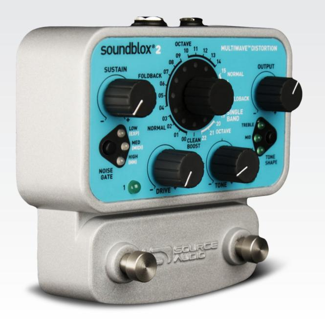
front of my Marshall. I found it lets you add some grit and compression in there, plus eq, making it do nice things in front of a crunchy valve amp. This pedal also has a compressor pot marked Sustain, which is a fantastic addition, opening up a whole world of tones with each of the distortion presets.
